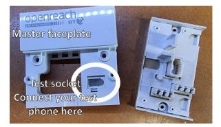
To verify whether a fault is internal or external, you need to remove the lower faceplate as shown in the pic. If your faceplate has another socket (RJ11) which connects to your broadband router, you should disconnect it as well.
